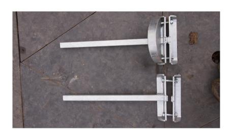
Next assemble the sawmill legs. Take the leg, and bar clamp and bolt it together using the M10 Bolts with nylock nuts. One side will also require the bar guard which goes on the top side protecting you or others from the protruding bar. Fit the bolts loosely for now as you will not tighten them until the chainsaw is in the mill.
