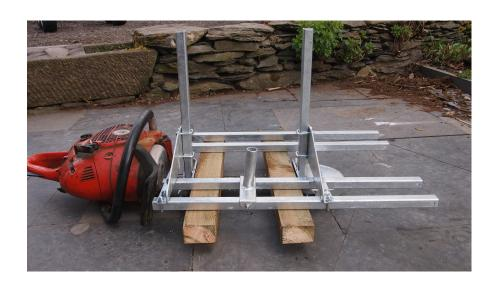
A handy way to set the depth is using some material the same thickness as you want to cut. Simply place the material in between the sawmill bars and your chainsaw bar, then tighted up the U bolts holding the legs to the mill. This avoids the need to use a tape measure and set up each end independently, and it is very accurate.
